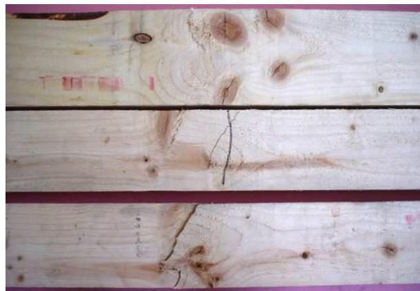
Figure 7. Machine grader rejects with severe cross grain.
