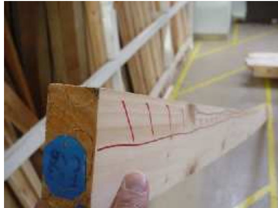
Figure 3. Distorted batten, originating from relatively straight log. (compression wood shown marked)
