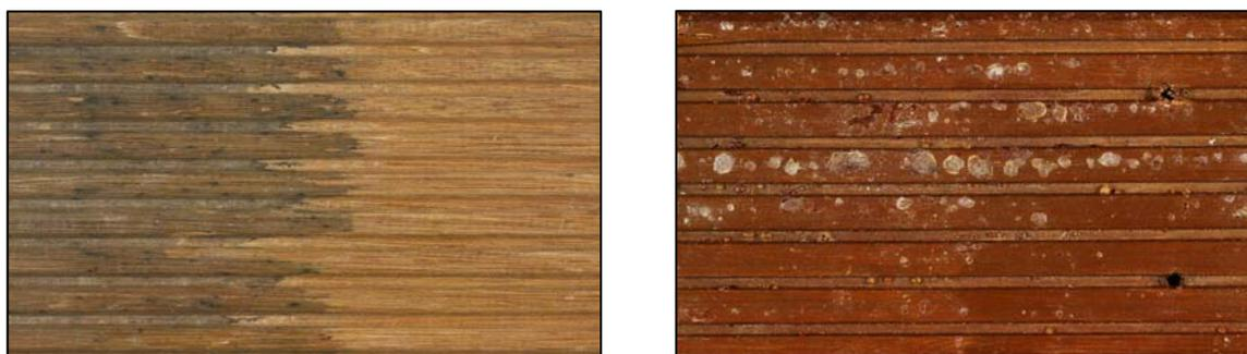
**Figure 6: Discoloration of bangkirai caused by a contamination with iron (left) and accumulation of resins on the wood surface of keruing (right)**
