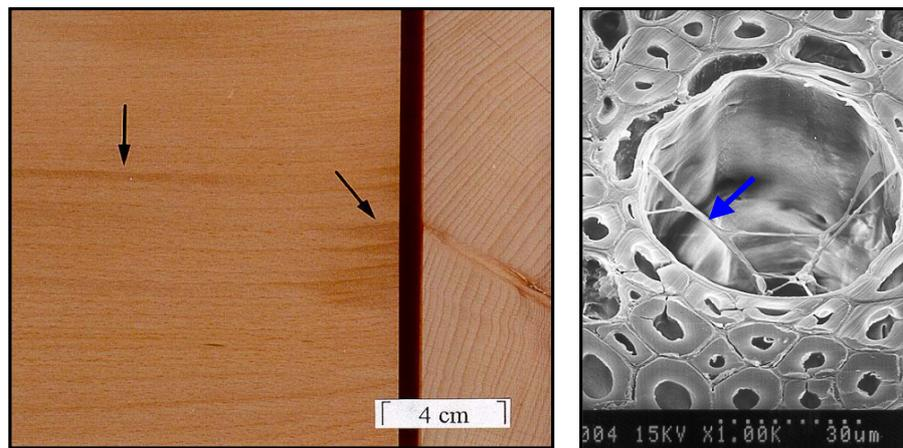
**Figure 3: Fungal stain on the wooden surface of steamed and not sufficiently ventilated sawn beech wood (*Fagus sylvatica*)**
