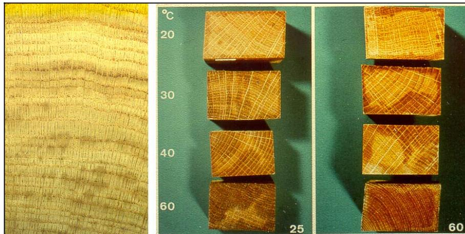
**Figure 5: Brown staining of kiln-dried oak. The discolorations are dependent on increasing kiln- temperature and relative humidity**
