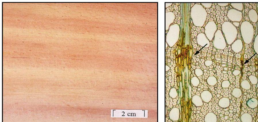
*Figure 2: Striped discolorations due to an inadequate storage of beech round wood. The discolorations are caused by physiological reactions of living parenchyma cells*
