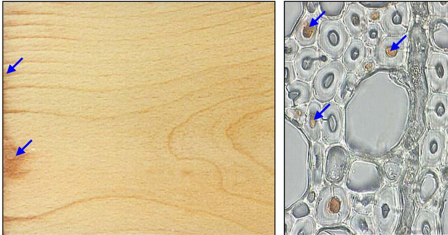
**Figure 4: Discolouration due to an accumulation of accessory compounds on the wooden surface of beech during the drying process**
